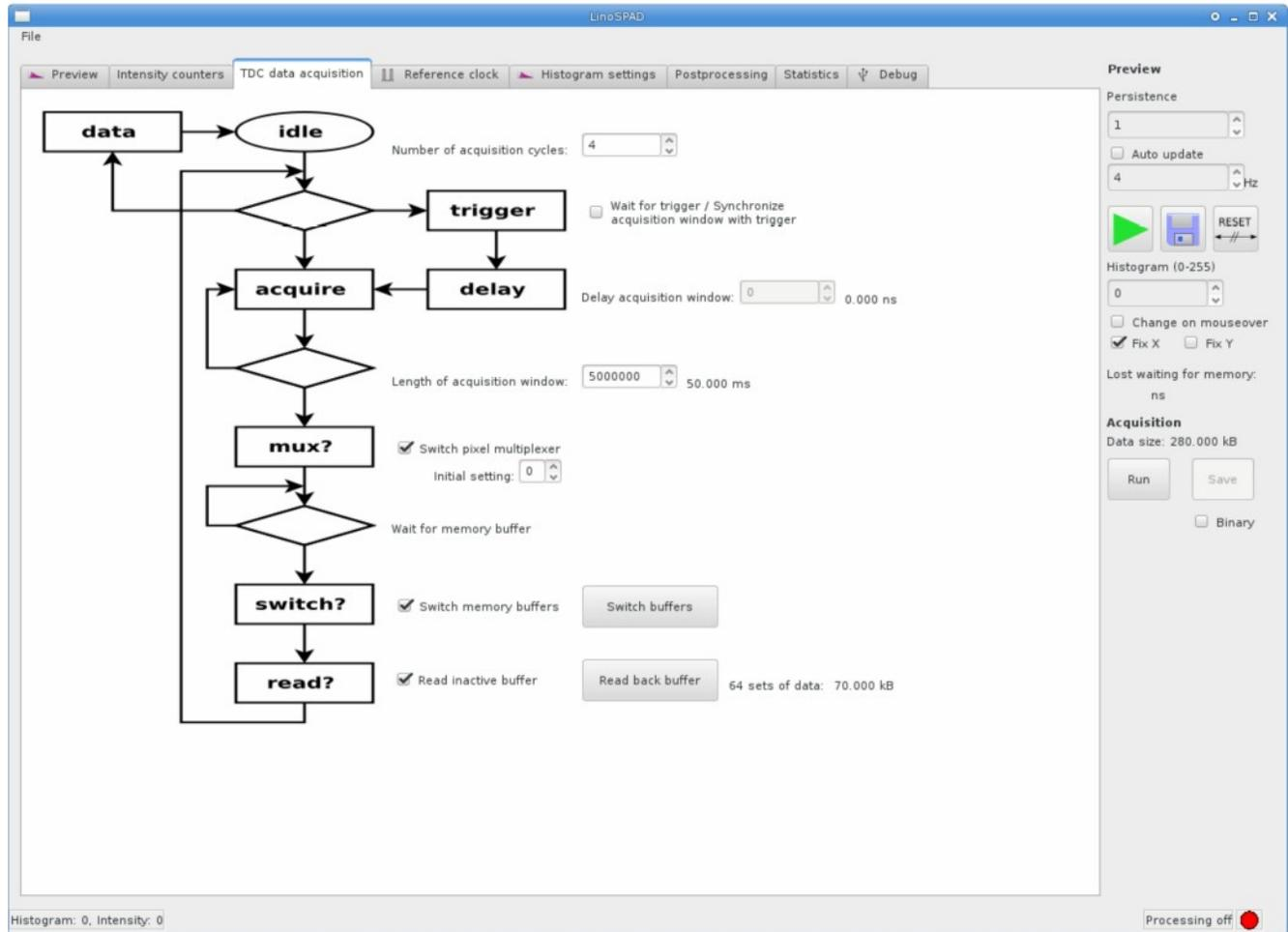
Figure 3: TDC data acquisition tab to control the acquisition window.
