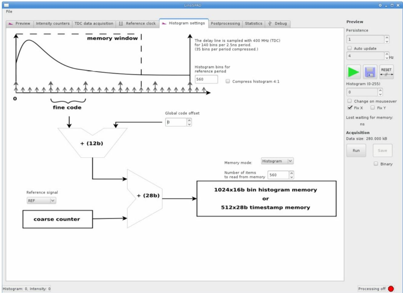
Figure 2: Histogram settings tab to select reference signal and memory mode.
