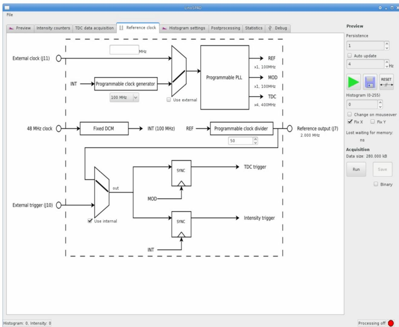
Figure 1: Reference clock tab used to control clock and trigger signals.
